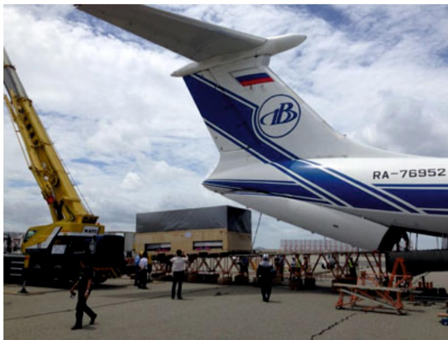
temperature environment below 30° C. To meet these requirements, the loading process in Sweden was performed early in the morning, standing time during the maintenance stop in Krasnoyarsk was reduced to a minimum, and the aircraft remained closed while the maintenance team installed equipment to unload the container in Japan. Additionally, Volga-Dnepr organised ground air conditioning unit to maintain the correct temperature,” added Alexey Stepanov.
