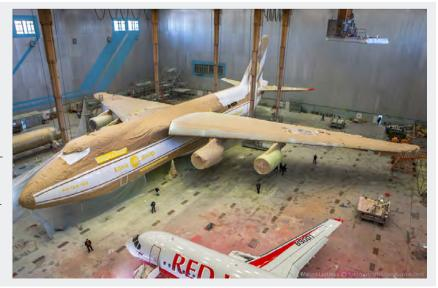
and this can be measured in terms of fuel savings. As a result of using the coating, we expect to cut the aircraft's fuel expenses by up to 1.5% or more than \$100 000 per year. The Base coat/clear coat system also gives a freshly painted look for a longer period so it also produces a saving in paint work too. The periods between washing of the aircraft can also be extended because the lacquer is more soil-resistant."
